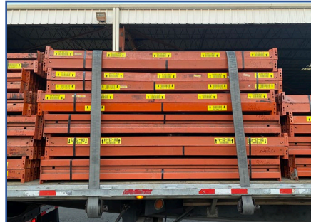
STICKERED Bundle all stickered beams together
